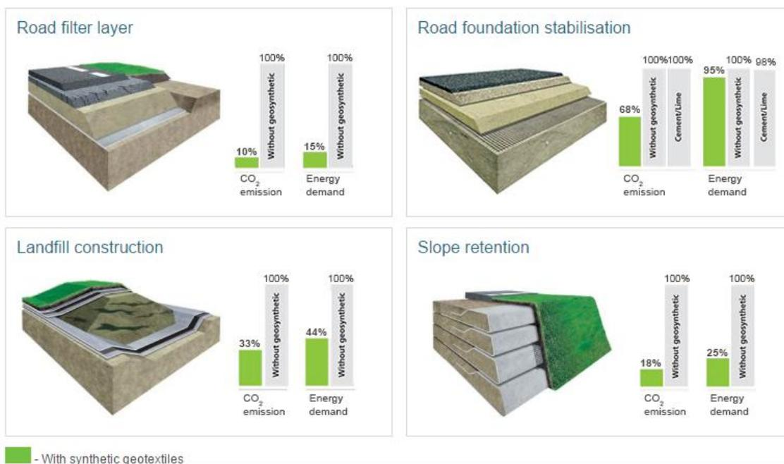
Figure 7. Summary of savings in CO<sub>2</sub> emissions and energy intensity structures in % with and without the use of geosynthetics.
