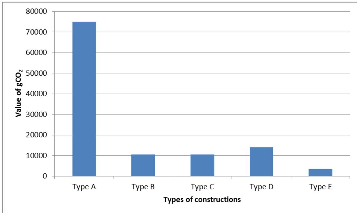
Figure 2. The value g of CO<sub>2</sub> in the extraction and production of raw materials and products of different types of terrace / retaining walls.
